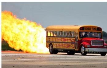
The bus can reach 357mph by using a 42,000HP engine from a McDonnell Douglas F-4 Phantom fighter jet. Photo: CATERS
